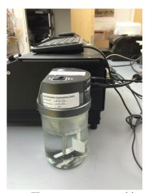
The new simulator directly connects to the side panel of the DMT via the air ports. The temperature cable connects to the DMT via an RS232 cable which is a small port on the simulator head and a large connection at the rear of the DMT. This simulator also has an on/off switch on the top. Software protocols (RPC and Simulator Solution Change) and maintenance procedures remain the same.
