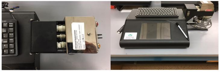
The old simulator connected to the DMT via a tower with locking arms. The simulator head contained connections for the air flow and the temperature.
